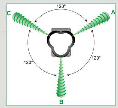
SODAR Transmits high frequency acoustic pulses and measures how they scatter and return. Sources of scattering are irregularities in wind velocities, air temperature and density, causing acoustic refractive index changes. By measuring the Doppler shifted frequency of the returned signal, wind speed and direction at various altitudes are determined.
