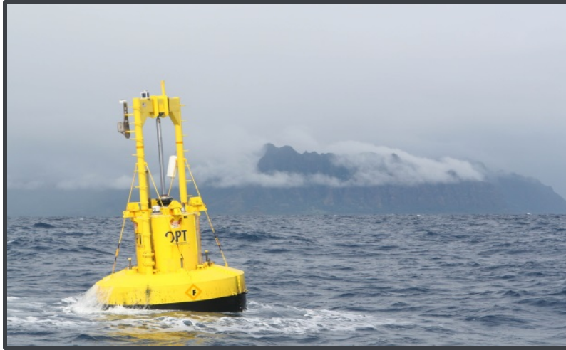
Ocean Power Technologie Test s Power Buoy at Navy Wave Energy Site, HI
