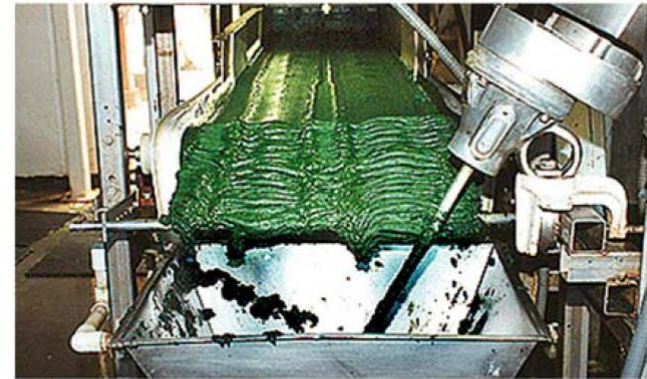
Fig. 5. Microalgal biomass recovered from the culture broth by filtration moves along a conveyor belt at Cyanotech Corporation ( www.cyanotech.com ), Hawaii, USA. Photograph by Terry Luke. Courtesy of Honolulu Star-Bulletin.
