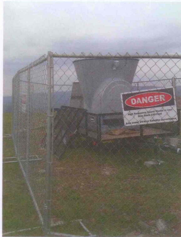
Bottom View: Close-up View of SODAR on Utility Trailer with Security Fence
